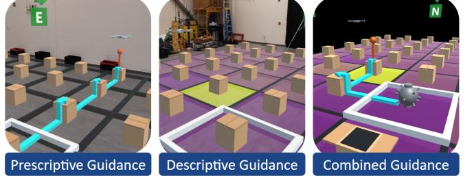
Fig. 2. AR-based visual guidance: prescriptive guidance - arrows and pins (left), descriptive guidance - an environmental heatmap (middle), and a combination of both (right) in an Minesweeper-inspired domain
