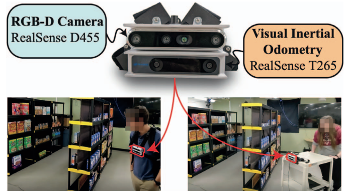
Fig. 5: ShelfAware hardware. A lightweight two-camera system with a 3D-printed mount was used throughout our experiments (top). This design allowed evaluation across a wearable chest mount (left) and a cart-mounted setup (right).
