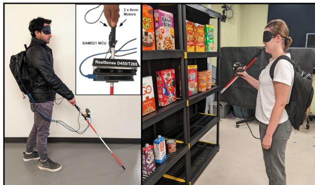
Fig. 1: Our system includes a robotic cane equipped with RealSense D455 and T265 cameras. The system is powered through a laptop in the backpack. *Left*: The system used as a navigational device. It used audio and haptic feedback for navigation guidance. *Right*: The system used as a manipulation device. It uses audio for manipulation guidance.
