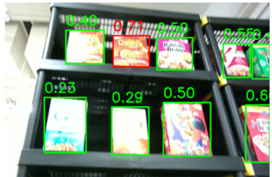
Figure 8: A sample product detection result that was robust to blurring and overexposure with the help of data association.
