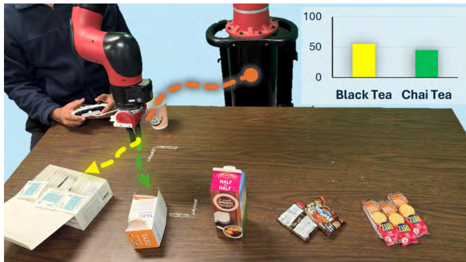
(a) Baseline setup. Without workspace optimization, the robot struggles to accurately infer which tea bag the user intends to pick up, leading to ambiguous goal predictions.
