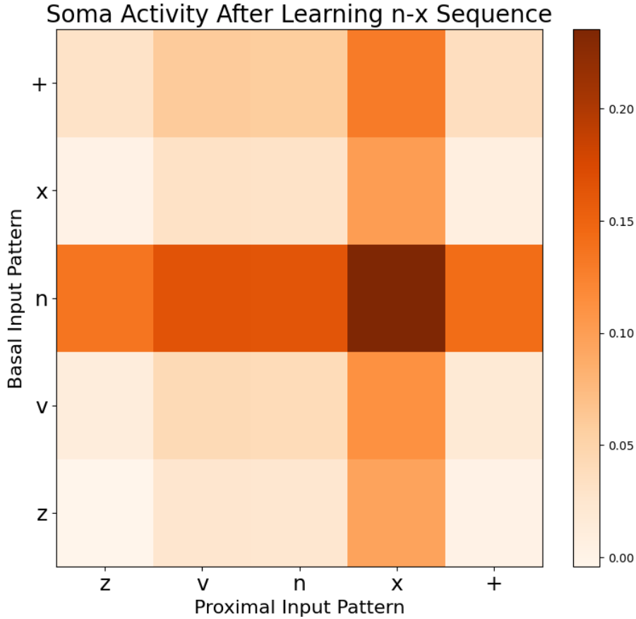
Figure 3.4: Signal in the soma for an n - x trained neuron given different input sequences. Each grid cell here corresponds to the average excitatory flux at the soma of a basal-proximal SOEN neuron. Basal input is received first, with a total of five pattern-specified input synaptic events, followed by five proximal input events. This is after learning the n - x sequence with the arbor update rule in only 7 training epochs. The correct ordering of input events indeed results in the most somatic activity and also the most output spikes.
