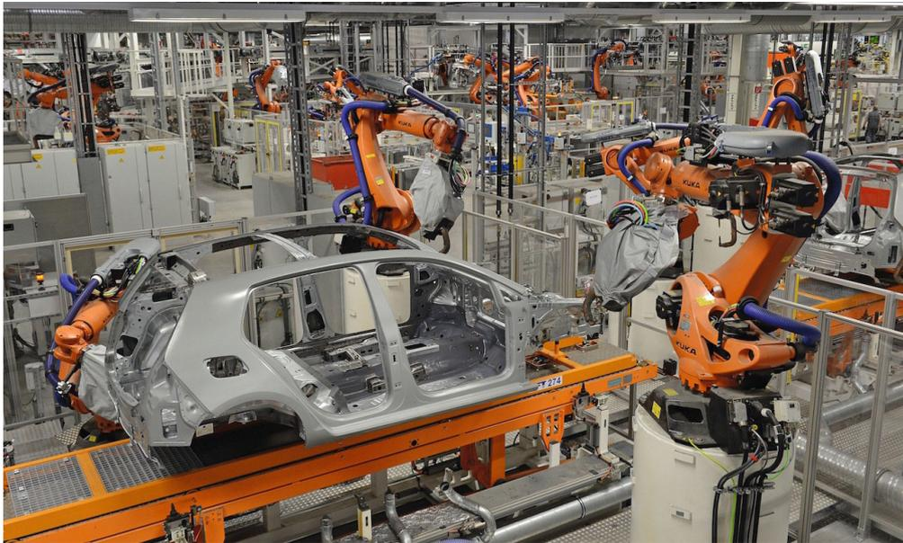
Figure 1.2: Robotic manipulators assembling a car in a structured factory setting. Image borrowed from [3].
